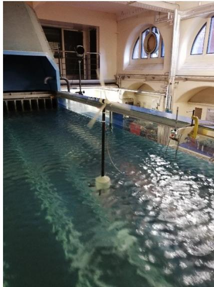
*Figure 2: Offshore wind turbine model placed in the WWC Tank at the Newcastle University*
